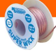
Any place you can put solder in, you can take it out with SUPER WICK. Remove the most expensive circuitry with confidence. Just lay the SUPER WICK on the soldered joint, apply tip of soldering iron to top-side for one second, and lift iron and SUPER WICK together to leave a clean connection ready for component removal or replacing. SUPER WICK is pure copper, specially woven wound on a pocket size spool with pressurized periphery.
